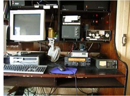
PMBO corner. The HF radio and Pactor modem can be seen above the mouse pad. Behind is a speaker and antenna tuner and to the left is the main computer.
